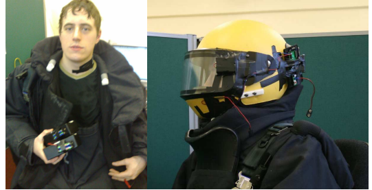
Figure 1: Explosive Ordnance Disposal (EOD) Suit with instrumentation
